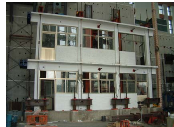
Laboratory Full Scale Cyclic Test 國家地震工程研究中心 National Center for Research on Earthquake Engineering
