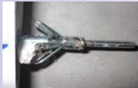
Punching Shear Failure
