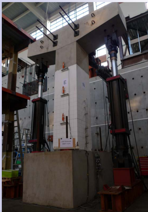
Tests of columns with high performance steel energy dissipation bars
