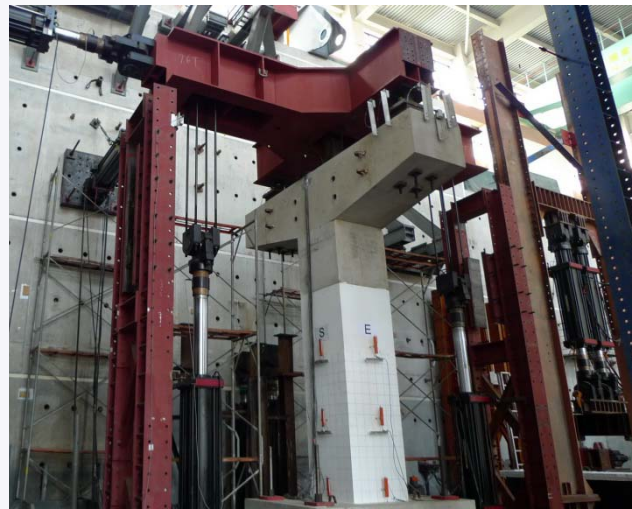
Tests of columns with lead-rubber seismic isolation bearings
